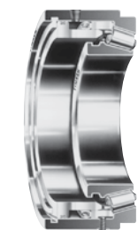
Fig. 108. Hydra-Rib bearing with preload adjustment device.
